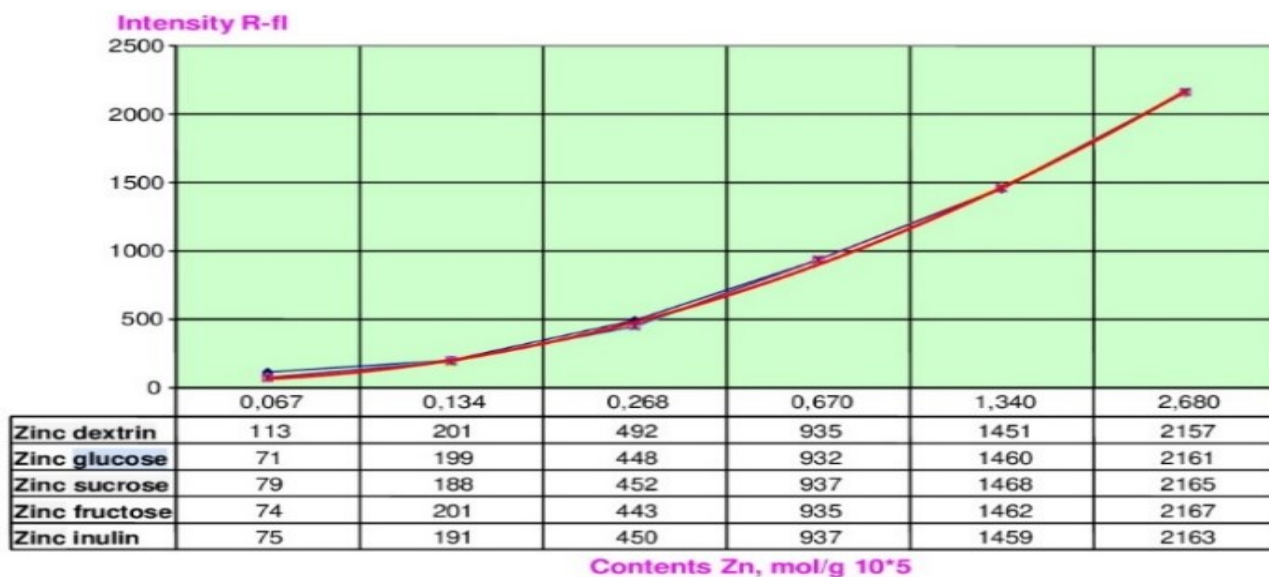
Figure 2. Determination of zinc content by X-ray fluorescence analysis using carbohydrates
