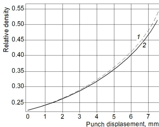
Figure 10. Change in relative densities of a tablet produced by double-sided compression: 1 – relative density at the core (centre) of the tablet; 2 – average relative density of the tablet
