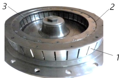
Figure 2. Working chamber of rotary pulsed apparatus
