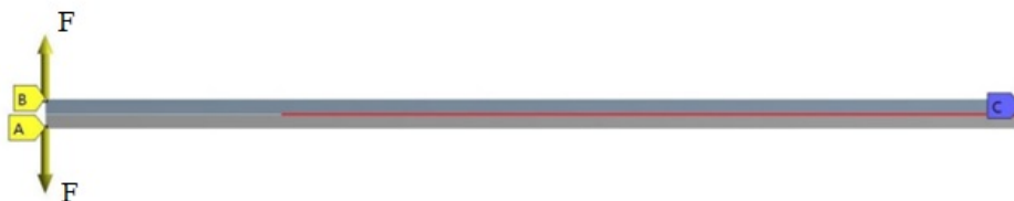
Figure 2. Finite element model of specimen bonded with hot-melt adhesive
