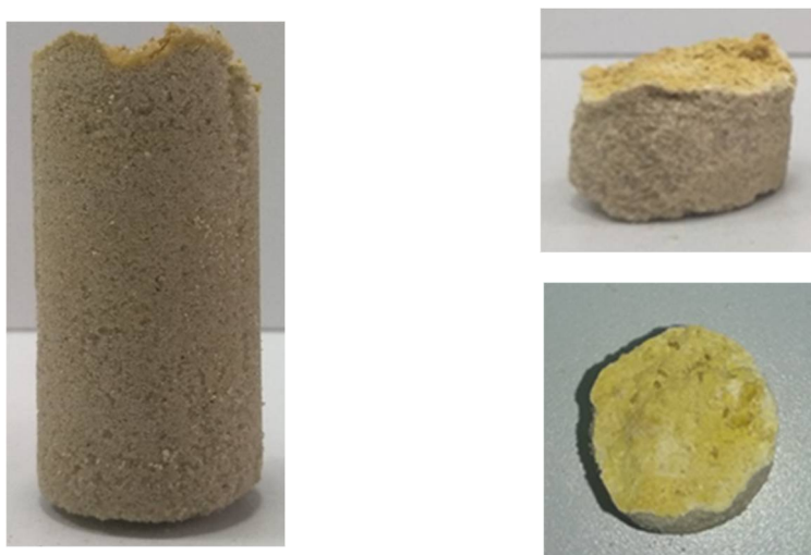
Figure 5. Sand after biocementation using soybean seed urease
