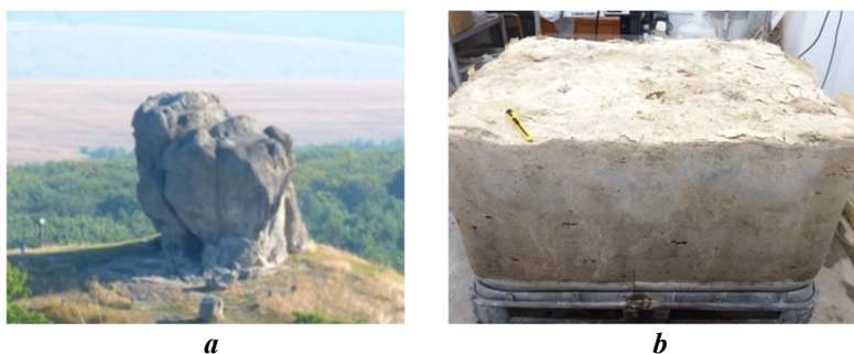
Figure 1. Object of natural biocementation: the rock in the village of Podkamin, Ukraine (a) and the result of artificial biocementation using MICP of sand (b)
