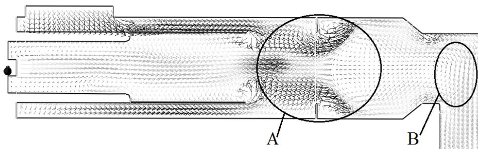
**Figure 8. Velocity vector gas streams after modernization**
