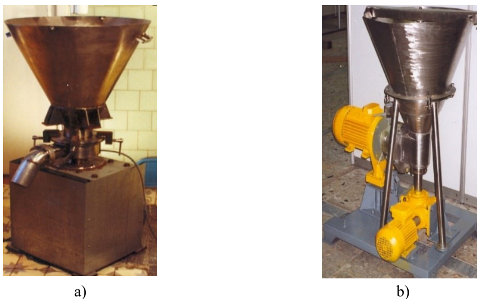
Figure 1. Rotary-pulsation apparatuses of cylindrical type developed at the IET NASU: a) model BGT; b) model BG-3
